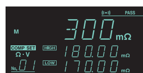
Resistance comparator value setting
