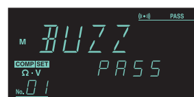
Buzzer mode setting
