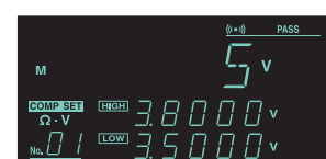
Voltage comparator value setting
